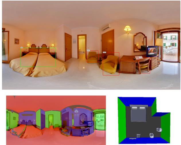
Figure 1: **Example output:** Indoor scene reconstruction from a single panorama image. Top: input image with 2D object detection bounding boxes. Detection is carried out in perspective images and the bounding box coordinates are projected into the panorama image. Bottom left: estimated surface orientations. Bottom right: reconstructed 3D room geometry and furniture items (top view).
