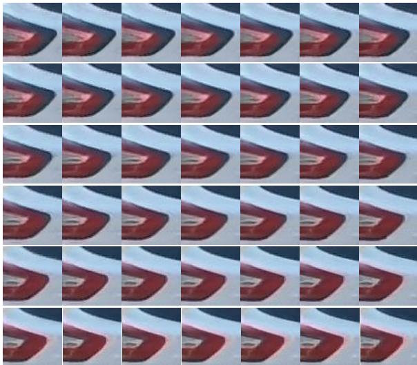
Figure 7: Example of interpolation of subtle motions. 42 frames (from left to right, top to bottom) are extracted by the proposed method based on the input image shown in Fig. 1. Please check the movement of the rear light comparing the first frame with last one. Note that there are no 42 original frames as the input blurry frame is produced by averaging only 7 frames. By iteratively applying the model we are therefore able to create slow-motion videos from blurry images.
