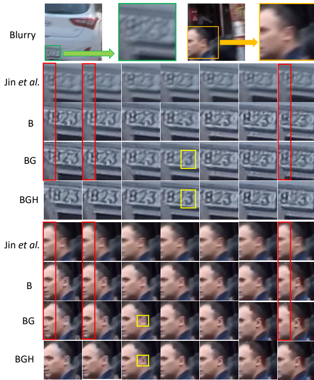
Figure 6: Qualitative comparison. Two input images and zoomed in regions are shown in the first row. The 2nd/6th rows show results of the method by Jin et al.[1]. The 3rd/7th to 5th/9th rows show the performance of our model trained after one (B), two (BG) and three stages (BGH). Note the movement across frames (referring to the fixed-position red boxes) is recovered successfully by the model BG, and the sharper detail inside the yellow boxes recovered by the fully trained BGH model.
