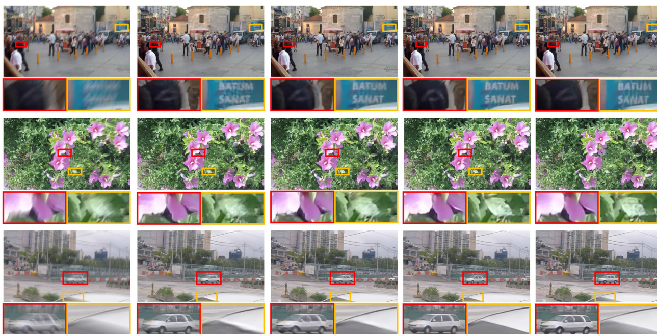
Fig. 12 Evaluation results of the state-of-the-art deblurring methods on the GoPro dataset Nah et al. (2017). From left to right: blurry images, results of Nah et al. (2017), Tao et al. (2018), DBGAN Zhang et al. (2020) and DeblurGAN-v2 Kupyn et al. (2019). Nah et al. (2017) and
