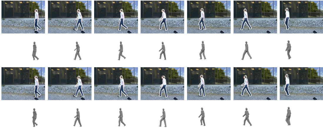
Fig. 7. Tracking a person walking fronto parallel to the camera . The first and second rows shows the frames from [16], overlaid with the body pose corresponding to the optimal path through the posterior distribution and the corresponding the 3D model, respectively. Similarly, second and third rows show the second best path. Notice that the second path describes the walk equally well except for the right-left leg flip which is one of the common ambiguity that arises in human pose estimation from monocular view. A total of 118 templates with 4 RVM mapping functions were used.
