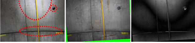
Figure 2: Sources of nuisance variability. From left to right: new query image with no relevant change; warped matching image from database; absolute difference image. The circled areas highlight significant nuisance variability.
