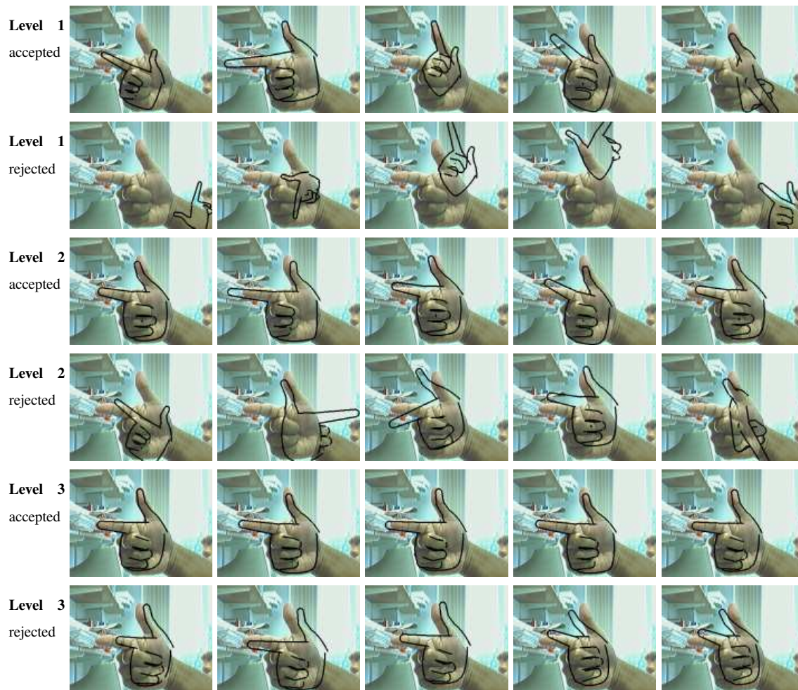
Figure 6.9: Search results at different levels of the tree. This figure shows templates above and below the threshold values \tau_t^l at levels 1 to 3 of the tree, ranked according to their posterior values. As the search is refined at each level, the difference between accepted and rejected templates decreases.
