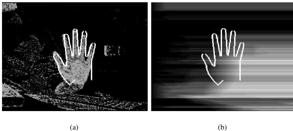
Figure 5.12: Efficient evaluation of colour likelihoods. (a) The skin colour log-likelihood image encoded as a greyscale image. Higher intensity corresponds to higher likelihood of skin vs. non-skin colour. (b) The sum table contains the cumulative sum of values in image (a) along the x-direction. The sum of values in within an area can be efficiently computed by adding and subtracting values at silhouette points only. The greyscale intensities are scaled to the range [0,255] in both images.
