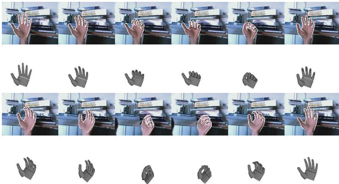
Figure 6.14: Tracking a hand opening and closing with rigid body motion. This sequence is challenging because the hand undergoes translation and rotation while opening and closing the fingers. 6 DOF for rigid body motion plus 2 DOF for finger flexion and extension are tracked successfully.
