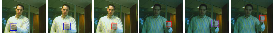
Fig. 12 Hand tracking using NCC-CM-M observers in parallel. The NCC observer (blue) is used initially. During motion blur the tracker switches to the CM observer (red). For a couple of frames the M observer (purple) is used, while the light is turned off, before switching back to CM.
