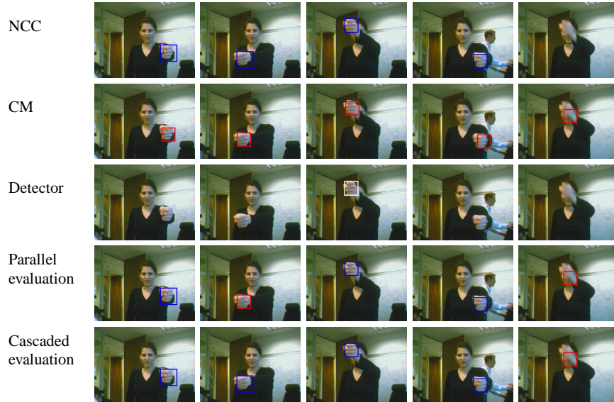
Fig. 11 Hand tracking results using NCC and color-motion (CM) observers. Shown are results of individual observers, a detector and parallel and cascaded evaluation. Colors indicate which estimate is used. In this sequence the hand is tracked successfully by both pair-wise schemes with a lower error than with either of the observers.
