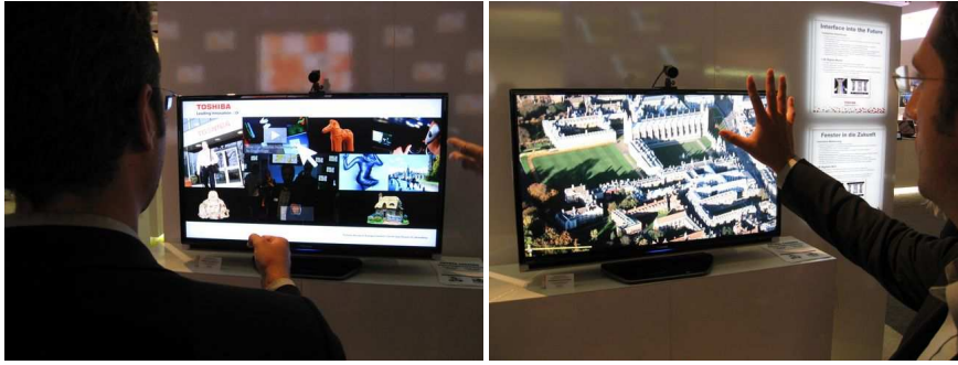
Fig. 1 Showcase of the proposed gesture interface. (Left) A single camera on top of the display is directed towards the user, who is able to control a screen cursor with his fist. Videos can be selected by hovering over a button. (Right) The playback of a video can be stopped with an open hand gesture.
