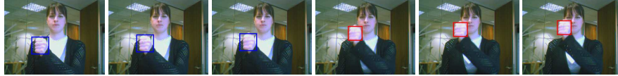
Fig. 13 Hand tracking using NCC-CM-FF observers in a cascade. The NCC observer (blue) is used initially, switching to the CM observer (red) during motion blur.
