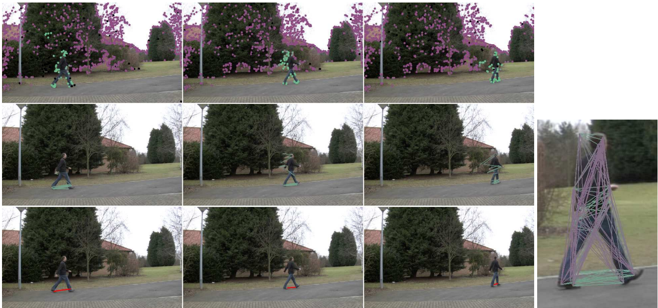
Figure 7. Results on Sequence I. Detection results superimposed on the input frames (from left to right, 150 frames between each view). Top: Extracted corner points and candidate points after the first stage are shown in green, the rejected points in purple, and points with trajectories of insufficient length in black. Middle: Pairs of corners extracted as feet in the second stage shown as green line segments. Bottom: Final detection after running mean-shift. Right: Example of all possible pairs between pre-selected corners at stage 1. Purple line segments are those rejected in stage 2.
