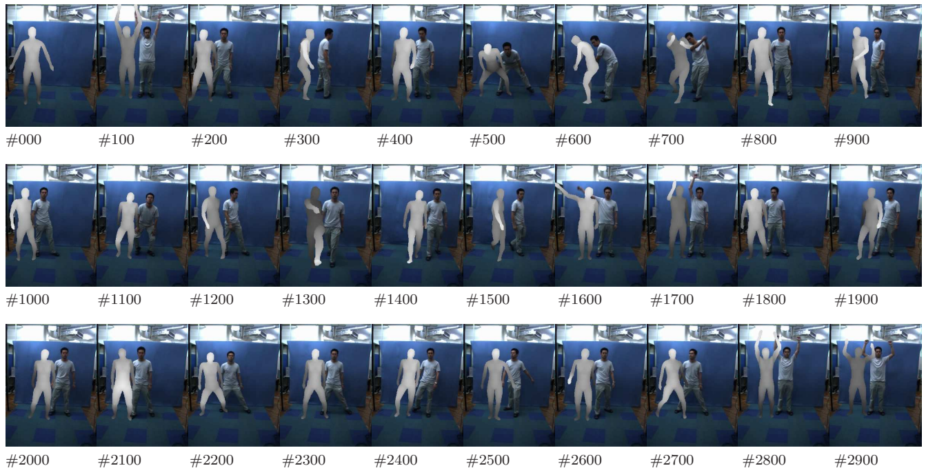
Fig. 8 Tracking results. The 3D model in the estimated pose is superimposed onto the input image with an offset. Our system recovers from misestimation occurring in frames #1300 and #1500. In these cases the likelihood values based only on the silhouettes is very similar for multiple poses.
