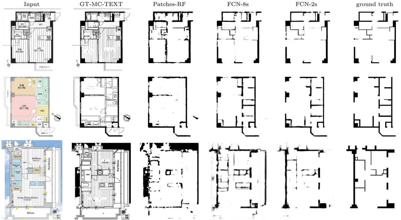
**Figure 3: Wall segmentation on images from the new R-FP data set.** Global thresholding (*GT-MC-TEXT*) does not handle decorative lines and symbols. The patch based segmentation (*Patches-RF*) cannot handle different drawing styles with the same parameter settings. Segmentations by *FCN-8s* [14] are more blurred than those by the proposed *FCN-2s*. The bottom row shows difficult example on which all methods perform poorly.
